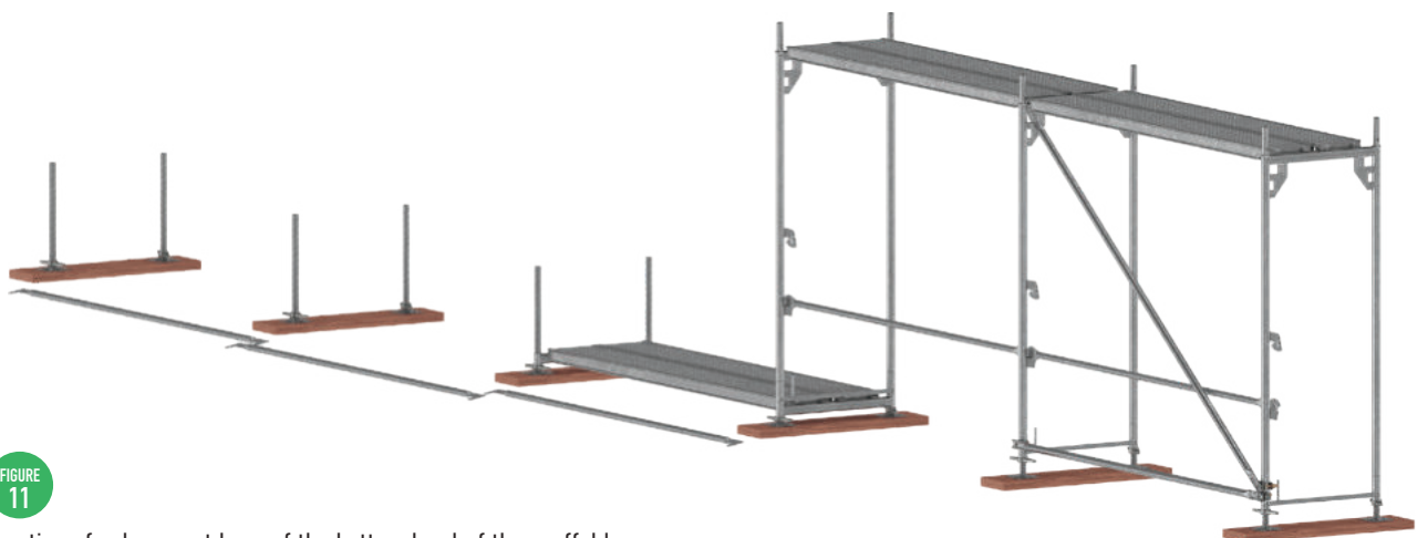
Erection of subsequent bays of the bottom level of the scaffold
